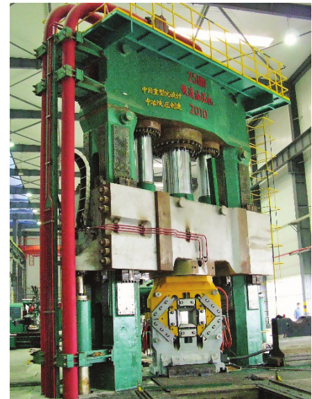
Application of a four-die forging device on a 25MN- and a 45MN presses (China)
