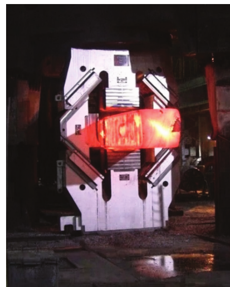
Forging a square section forging in FDFD on a 30 MN press (Japan)
