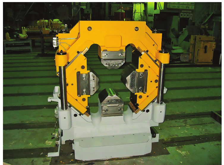
Four-die forging device with a spring employed to lift the top body for a 10MN press (Germany).
