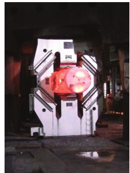
FFFD with dies for producing square forgings and with dies for producing round forgings on a 30 MN press (Japan)
