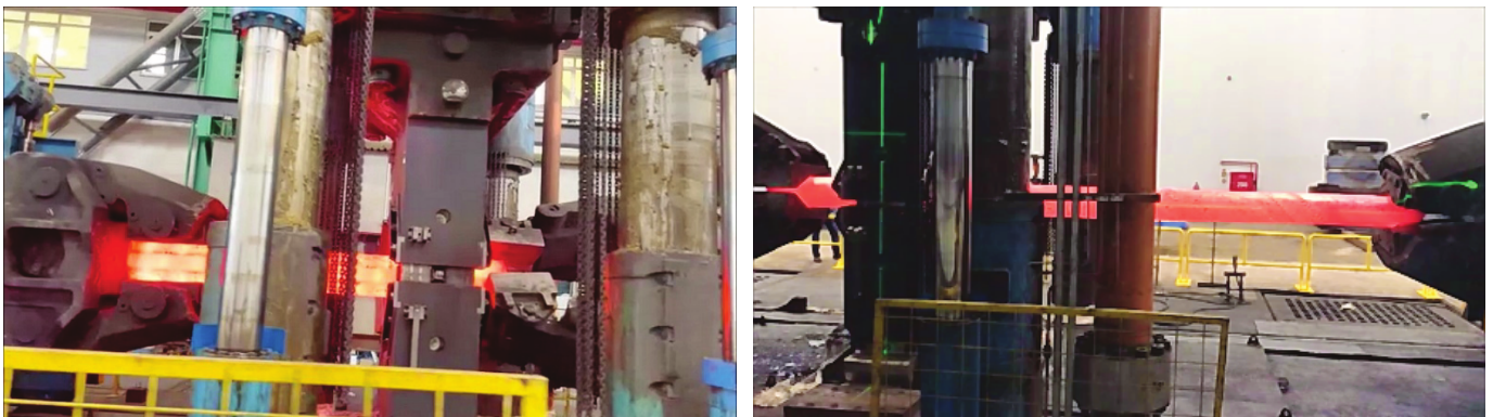
Forging in FDFD on a 40 MN press with two manipulators (Turkey)
